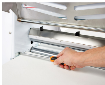
Facilitated replacement of the belts in under thirty minutes.
