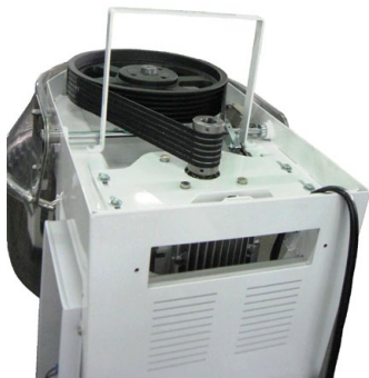
1 Toughness: power transmission by belt requires no maintenance
