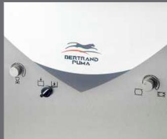
Pressure adjustment knobs, and full-tank and half-tank modes.
